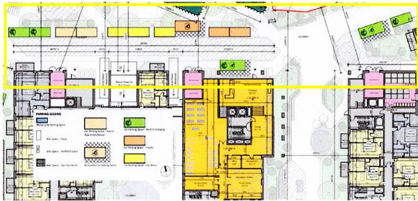
Fig. 45: Loading bay area for the scheme and the parcel room for the scheme are sited at Block 3
